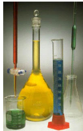
Volumetric glassware: a buret, a volumetric flask, a graduated cylinder and a pipet. (C. D. Winters)
